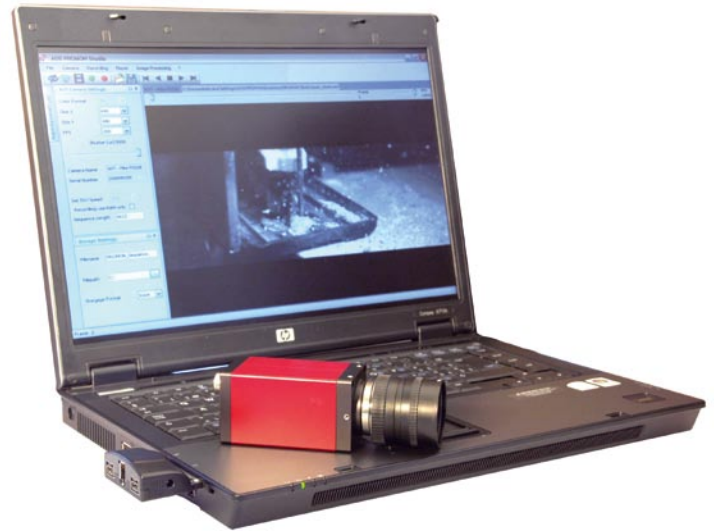
Laptop PC, camera and IEEE1394b interface (PCMCIA)
